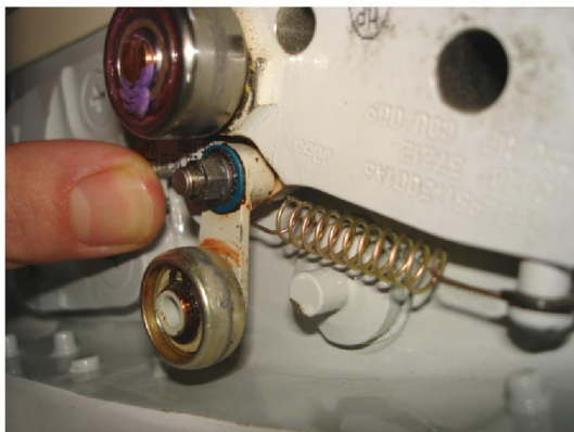
Figure 2: Installation of Safety Catch Spring
